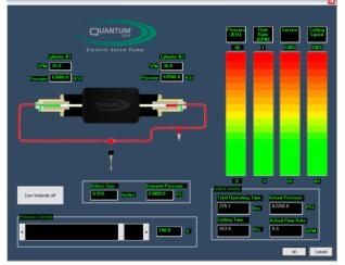
The Quantum ESP<sup>™</sup> software diagnostic screen gives a quick and easy-to-read analysis of the pump performance, with an in-time graphical representation of the relationship between pressure, flowrate, maintenance and cutting speeds. This will help the operator determine the correct set up for a given application.
