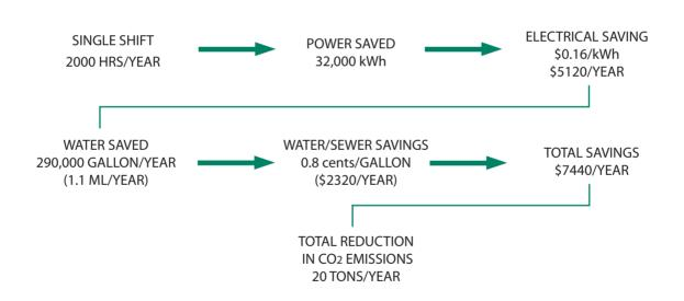
\*Note: If a recycling water chiller is used, the water savings will be \$0, however the power savings would increase from \$5120 to \$7360, as only a 3 kW chiller is required for the TECHNI Quantum ESP™.
